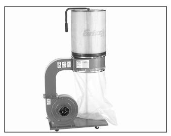
Figure 19. Lower collection bag installed.
